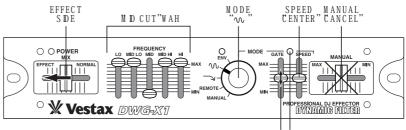
Adjust the GATE CONTROL to the degree of input source whether it's big or small You can make this setting precosely when LFO /DOWN indicator has flashed to the beat.
