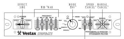
Adjust the GATE CONTROL to the degree of input source whether it's big or small You can make this setting precisely if you adjust GATE CONTROL, the ENVELOPE indicator lights up.
