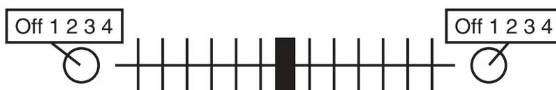
In this example "Hard left" selects Channel 1 and "Hard right" selects Channel 4. With the crossfader centred, both assigned channels are live. Use the crossfader for fast and seam less segues from one selected channel to the other.
