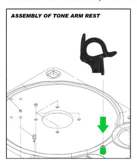
Serves to secure the arm against movement. Use during transport turntables. NOTICE: use caution when assembling.
