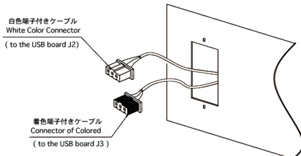
**3.** When you can verify that you connect to the J2 terminal and the J3 terminal just, in order in the type where the TUB-1 installation hole becomes depth for the LED indicatory lamp to be above, it inserts in the installation hole, it locks with bis 2 you remove some time ago. In addition, when it is the type where the TUB-1 installation hole becomes wide, in order for the LED indicatory lamp to be left side, please install.
